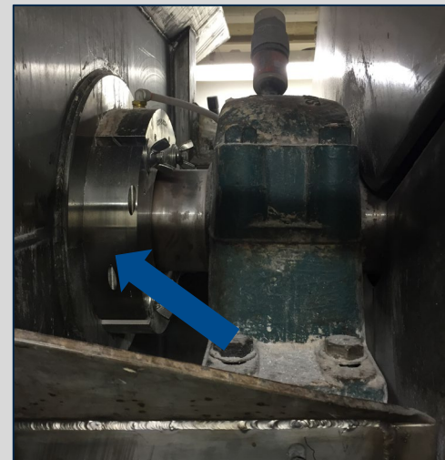
After: Inpro/Seal Food Grade Air Mizer shaft seal
