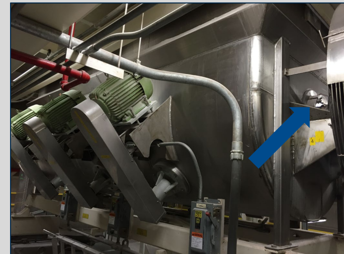
After: Inpro/Seal Food Grade Air Mizer shaft seal
